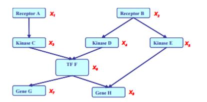
$P(X_{1}, X_{2}, X_{3}, X_{4}, X_{5}, X_{6}, X_{7}, X_{8})$   $= P(X_{1}) P(X_{2}) P(X_{3} | X_{1}) P(X_{4} | X_{2}) P(X_{5} | X_{2})$   $P(X_{6} | X_{3}, X_{4}) P(X_{7} | X_{6}) P(X_{8} | X_{5}, X_{6})$
