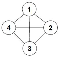
A fully connected graph with pairwise (edge) potentials on binary-valued nodes (for x<sub>i</sub> ∈ {−1,+1} or x<sub>i</sub> ∈ {0,1}) is called a Boltzmann machine
